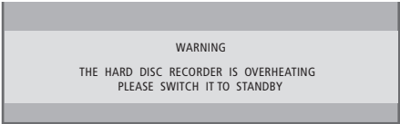
If this warning appears on the screen and you do not switch off the hard disc recorder, it switches itself off automatically after a few minutes, and remains off until it has cooled sufficiently. You cannot operate the hard disc recorder during this time.
